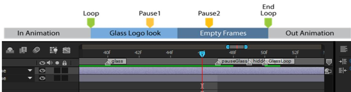
**Real-time DVEs** leverage the creation of animated objects to represent the scaling and position used in squeezeback events. A designer has full control over not only the attributes of the DVE boxes, but also of the other graphic elements that can be interacting with the rate and position of the squeeze. This DVE information is then forwarded to the Versio Graphics playback engine, which executes the exact same operations in real time to the switched live or clip sources.
